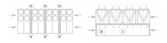
Air intake: 2 front sides over the entire height; up to 10 units; Minimum distance  $A_{\mbox{\scriptsize min}}$  between two units:
