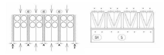
Air suction: 2 front sides over the entire height; up to 10 units; Minimum distance  $A_{\scriptscriptstyle min}$  between two units:
