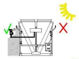
Install the supplied sensor in a shaded location.
