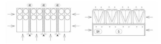
Air suction: 1 front side and 2 side over the entire height; up to 10 units; Minimum distance  $A_{\tiny \mbox{min}}$  between two units:
