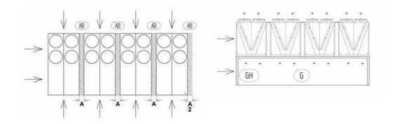
Air suction: 2 front side and 1 side over the entire height; up to 10 units; Minimum distance  $A_{\tiny \mbox{min}}$  between two units:
