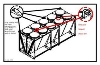
40 - "Lifting and anchoring point" notice
