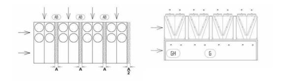
Air intake: 1 front side and 1 side over the entire height; up to 10 units; Minimum distance  $A_{\text{min}}$  between two units:
