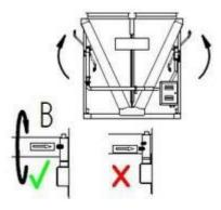
Twist the pipe upwards until the marking lines are positioned next to each other (B).
