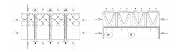
Air suction: 2 front sides and 2 sides over the entire height; up to 10 units; Minimum distance  $A_{\mbox{\tiny min}}$  between two units:
