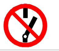
Fig. 2: Example for a warning sign when securing the machine against being switched on again
