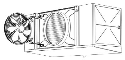
After cleaning the swivel fans must be put back to their original position and fixed and secured here against unintentional or unauthorised opening.
