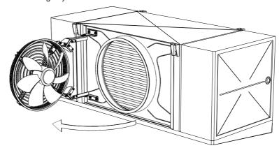
Ensure that units with electric block defrosting have enough space for changing heater rods.
