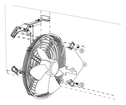
9. Fix swivel unit with pre-mounted fan on the bolts named under 3. NOTE! Tighten nuts hand-tight only!
