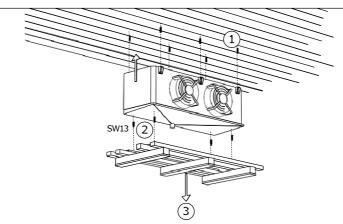
The units are delivered in the installation position.
