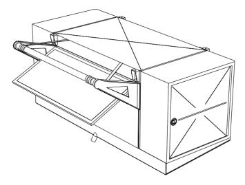
Fabric closure devices may only be used with use of fan ring heaters with reduced heating power and corresponding installation accessories.
