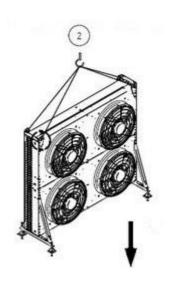
2. Screw the unit firmly to the ground. If used, mount the optional vibration dampers supplied (see the section "Mounting the vibration dampers (optional)").
