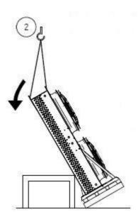
2. For easy mounting of the feet, place the unit on a level surface in order to avoid damaging the fins. The height of the surface must be at least as high as the length of the legs.
