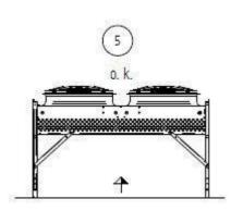
5. Once again, check all screw attachments. If used, attach the optionally supplied vibration dampers.
