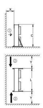
Floor installation; side view (above) and plan view (below)
