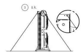
3. Attach bracing cables only to the eyelets provided. Position the bracing cables according to the specification of the static system.
