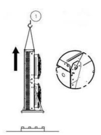
1. Lift the unit off the pallet and transport it to the installation site. Attach transport cables only to the crane eyes provided.
