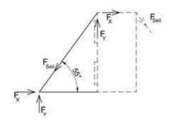
Cable tension:  $F_{cable} = 3.5 \text{ kN}$ Resultant forces:  $F_{x} = 2.1 \text{ kN}$
