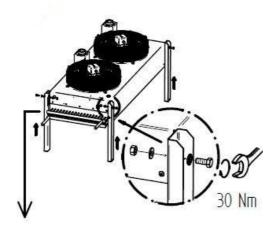
4. Screw the feet firmly to the unit.
