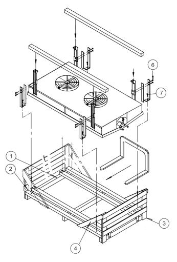
The palette then serves for lifting the unit (including mounted drip tray) when installing at the set-up point.
