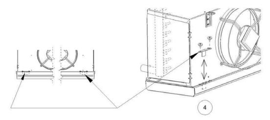
(4) Secure the drip tray with two retainers on the fan side. To do this, screw the retainers firmly into place using two screws and washers.
