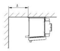
Minimum distance N: GACC 031: N = 375 mm GACC 040: N = 450 mm GACC 050: N = 550 mm
