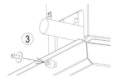
(3) Fasten the drip tray to the unit using two screws and corresponding washers.
