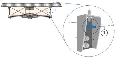
Ceiling fixing (as standard on the brackets).
