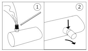
1: Check/release transport overpressure / 2: Remove blanking plugs.
