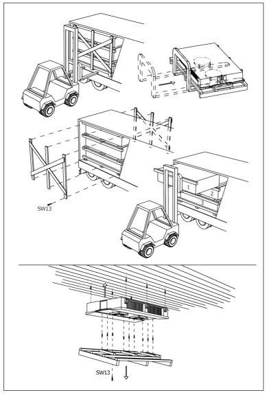
15, 17, 26 - Ceiling-mounted air cooler loading
